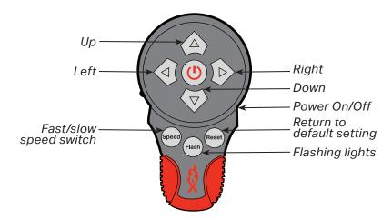
■ The Remote Spot Controller uses a 23A 12V battery.
