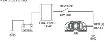
DO NOT wire in parallel with a sloenid or relay coil. DO NOT spray any coating material, e.g. paint, undercoating, etc., over the sound opening. DO NOT install the product or its wiring in proximity to ignition wires. Failure to observe these conditions may have an adverse effect on the product's performance.
