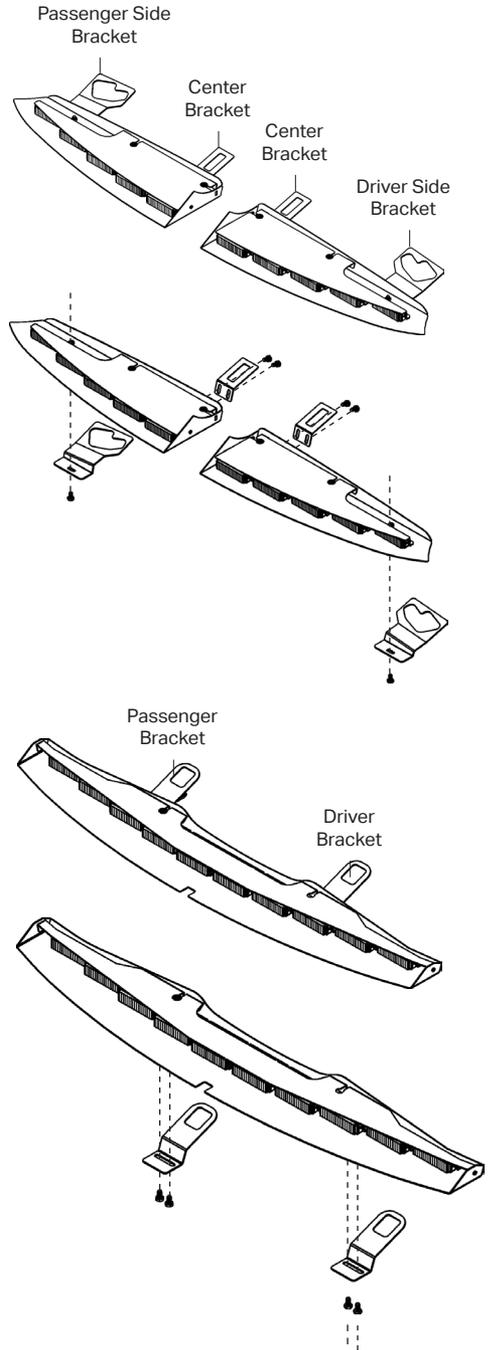
**Step 4:** With the light bar against the headliner and the brackets positioned, reattach the visor clips back into their original position using the original hardware.
