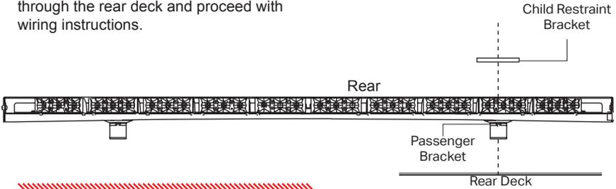
**Important!** Depending on vehicle, additional adjustments may be needed during installation, such as bending the visor clip brackets.
