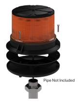
Using the hardware provided, secure the beacon to the pipe-mount adapter, feeding the wire down through the center of adapter plate. After making the appropriate wiring connections, feed the wire through the pipe and tighten the beacon onto the pipe. Tighten the adjustment nut to complete the installation.
