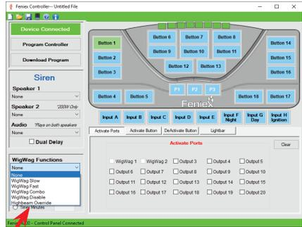
Program the appropriate input (high-beam signal) to override the flashing wig-wag function with a steady-on signal.
