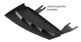
**1.** Mount the interior lightbar to the visor bracket in your vehicle. The front of the base should be flush with the windshield.
