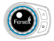
**Dim Mode:** Press the % button to cycle to Dim Mode (indicated by blue). Rotate the dial to adjust the brightness. When the led screen is completely dim, no lights will be on. When the led screen is completely lit, the bar will be at 100% brightness.
