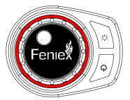
■ Focus Mode: Press the <sup>+</sup> button to cycle to Focus Mode (indicated by red). Rotate the dial to adjust the focus on the lights. When the LED screen is completely dim, the lights will be in full spread. When the LED screen is completely lit, the lights will be in full spot.
