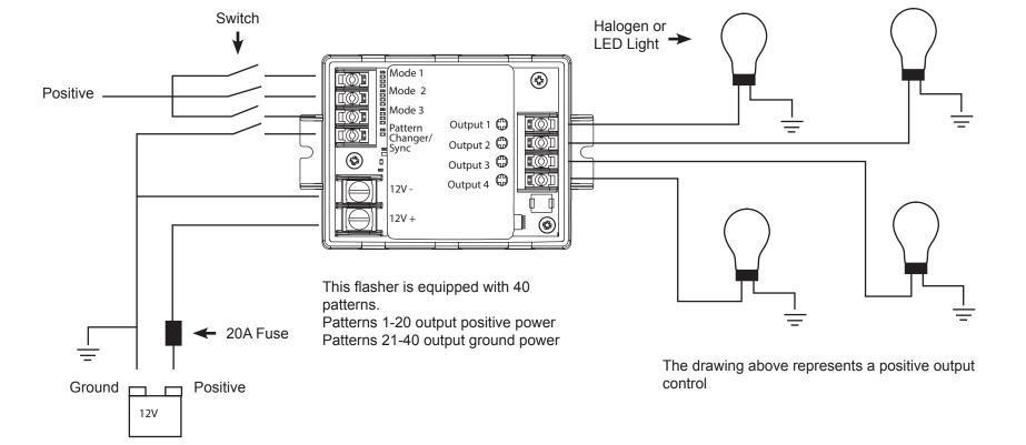
Flashing Red LED: 12V+ Output Control Flashing Green LED: 12V- Output Control
