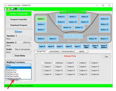
Program the appropriate input (highbeam signal) to override the flashing wig-wag function with a stead-on signal.
